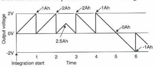
With the 1 A range selected, and the integration time set to one hour, in the case that +1 A is measured for 2 hours 30 minutes, and thereafter -1 A.
